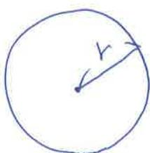
$$\text{area } A = \pi \times \left(\frac{C}{2\pi}\right)^2 = \pi \times \frac{C^2}{4\pi^2} = \frac{1}{4\pi} \times C^2$$
